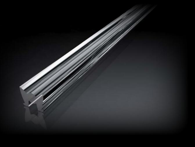
SLOT is a linear luminaire located behind – and shining through – a slot. The luminaire is linear in appearance. Individual points of light are not visible. The heart of the luminaire is a linear extrusion primary TIR lens with an exactly-positioned secondary lens. Slot is suitable for office workplaces (UGR < 19), thus requires longitudinal glare control. The primary optic provides transverse direction focus, the secondary optic longitudinal.
